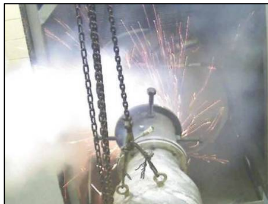
Figure 2: Burst during containment testing [2]
