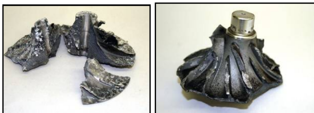
Figure 3: Hub burst and wheel detachment. [3]
